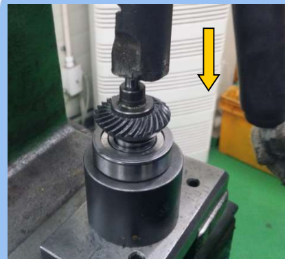
38) SPACER, BEARING(6204ZZ) 조립
