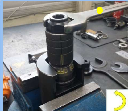
26) AIR INLET BUSHING 분해
