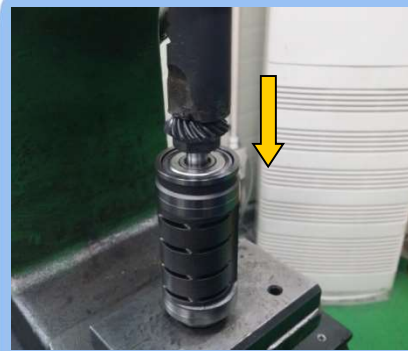
35) DRIVING GEAR 조립
