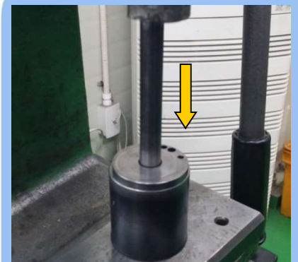
24) REAR PLATE BEARING(6001ZZ) 분해
