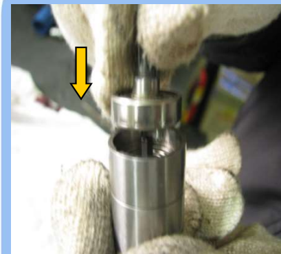
15)ROTOR PINION 조립
