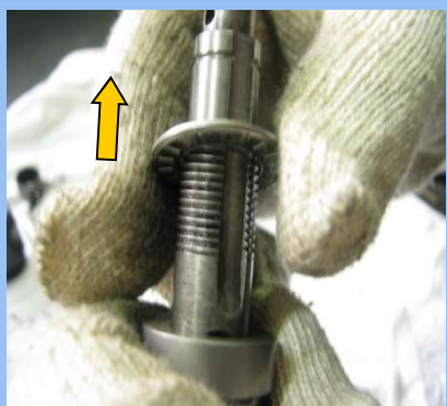
28)THRUST BEARING 분해
