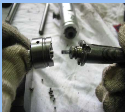
34) CAM CLUTCH와 SPINDLE CLUTCH 분해
