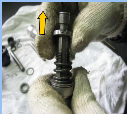
25)ADJUST LOCK PLATE 분해
