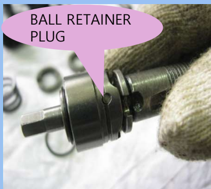
31) BALL RETAINER PLUG 분해
