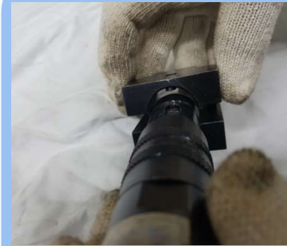
3)CLUTCH HOUSING 치구고정
