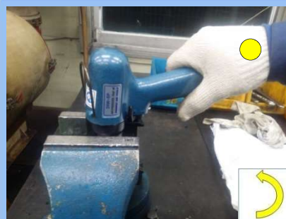
23)HAMMER CASING 조립
