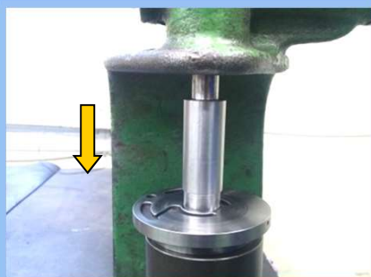
19)FRONT PLATE BEARING 분해
