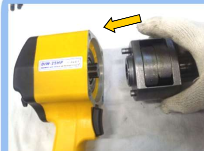
33)FRAME HAMMER ASSY 조립
