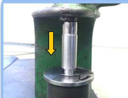
18)REAR PLATE BEARING 분해
