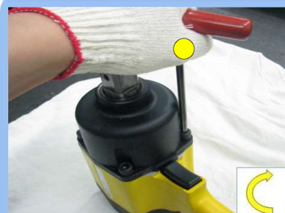
35)ALLEN HEAD BOLT 조립
