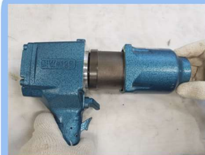
3) HAMMER CASING 분해
