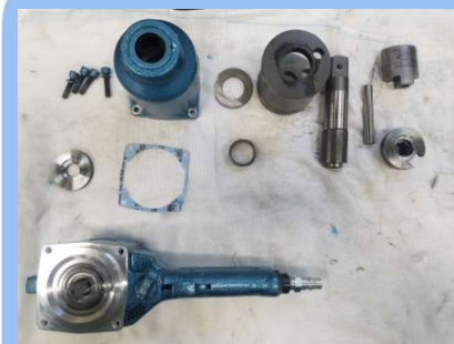
12) HAMMER CASING 분해모 습
