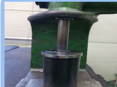
21) FRONT, REAR PLATE BEARING 분해
