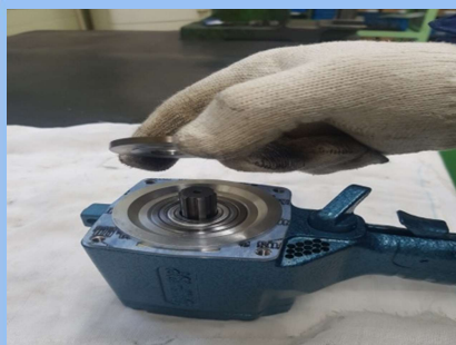
11) HAMMER CASING SPACER 분해
