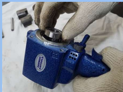
26) FRONT BEARING 조립
