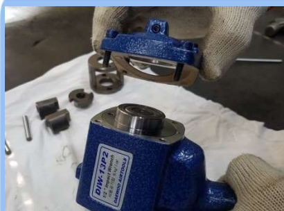
28) CASING COVER 조립
