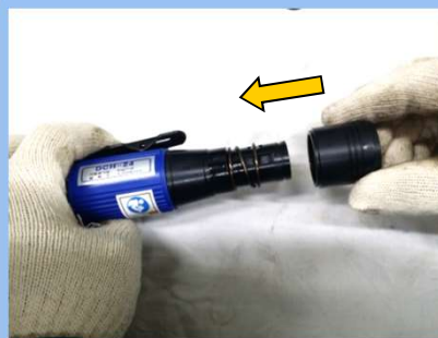
23)EXHAUST DEFECTOR 조립
