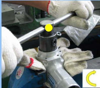
7) CASING FRONT COVER 분해
