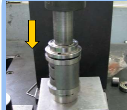
27) CYLINDER, FRONT PALTE, BEARING(629ZZ) 조립
