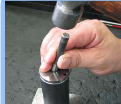
15) FRONT PLATE BEARING(629ZZ) 분해
