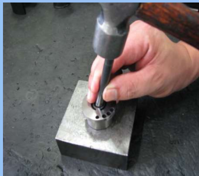
16) REAR PLATE BEARING(629ZZ) 분해
