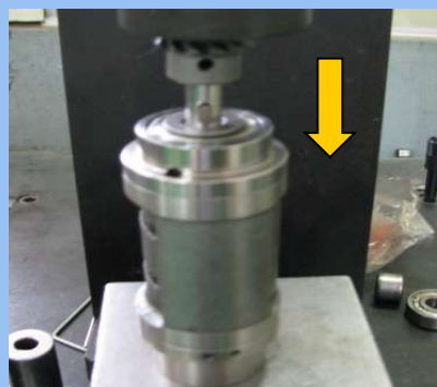
28) SPACER, KEY, DRIVING GEAR 조립
