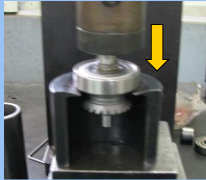
19) SPINDLE BEARING(6203ZZ) 분해
